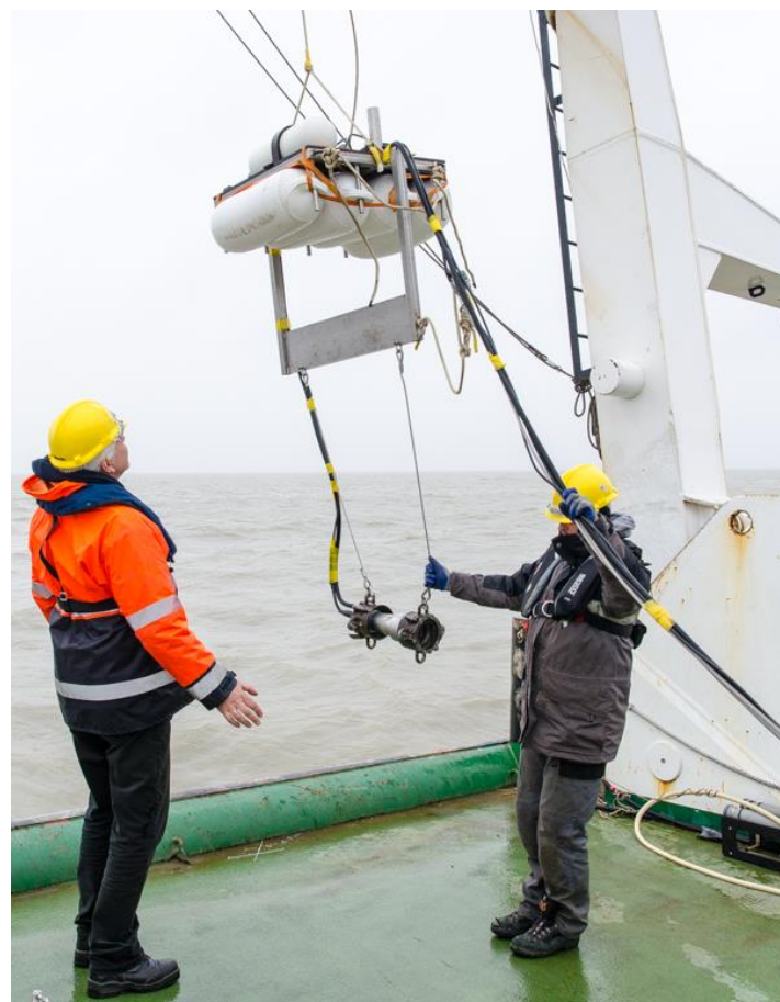
Figure 9 - Deployment of Sleeve gun and floating frame on RV Belgica.
