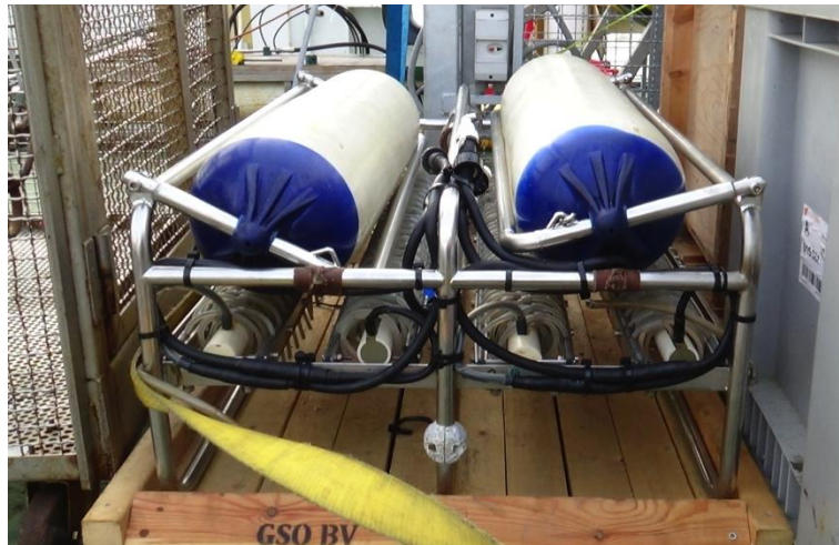
Figure 10 - GSO 360 tips sparker attached in its floating frame
