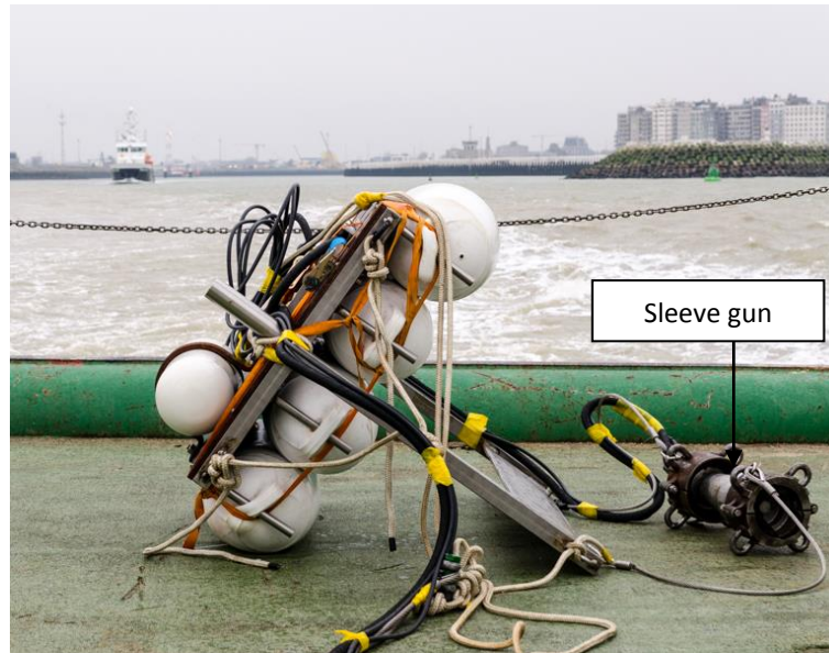
Figure 8 - Sleeve gun (on the right) on the deck of RV Belgica. On the left the floating frame can be seen.
